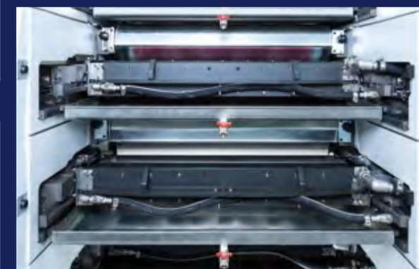
A solid design with 100 mm steel sideframes and outstanding stability as standard
