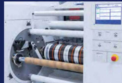
Turret style winders: Highly productive thanks to fully automated splices at production speeds of up to 400 m/min
