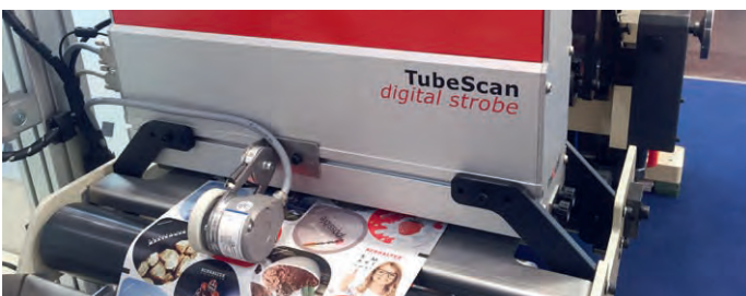
TubeScan reliably detects tiniest pinholes in yogurt lids
