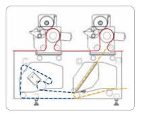
UV on chill drum UV/UV Led + Hot Air + Extendend path for UV coating
